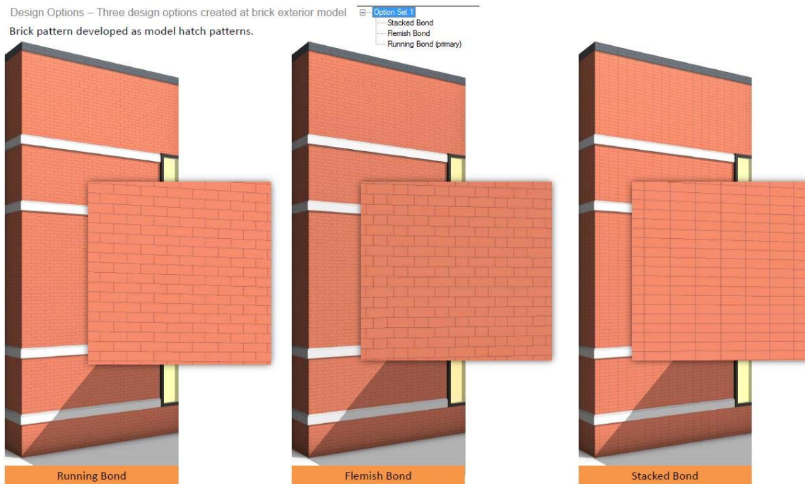
Figure 4-10. Design Options for Masonry Bonding Patterns (Rendering)
